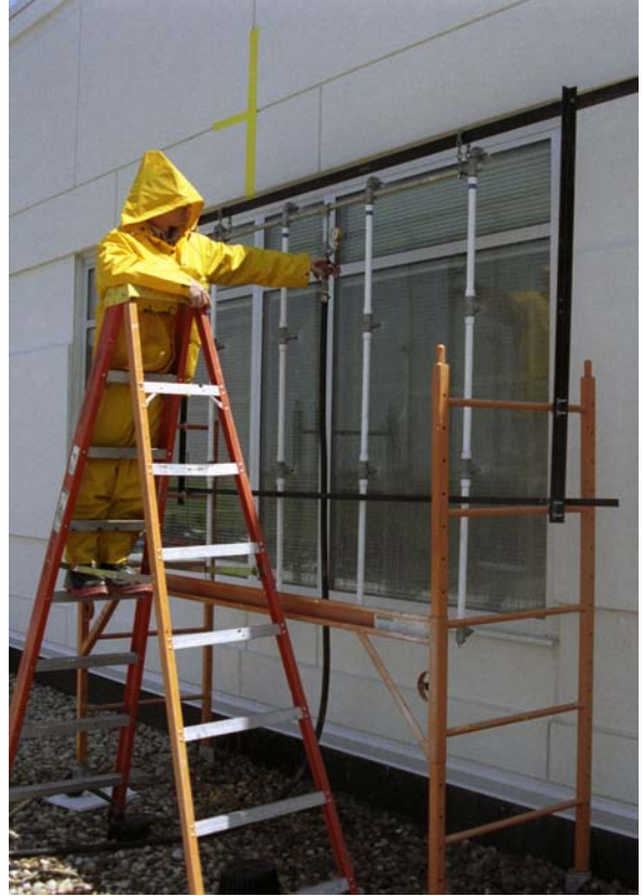
ASTM E1105 test for water penetration of windows
