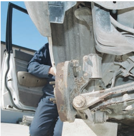
Suspension failure results in a fatal vehicle rollover
