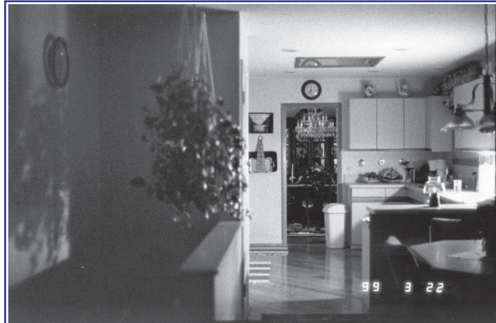
A woman spending the night in an unfamiliar place, turned left at the staircase and fell down the stairs, instead of walking straight through the kitchen on her way to the bathroom. The only illumination was the lamp over the sink in the kitchen. To determine visibility, it was necessary to recreate the lighting conditions as they were at the time of the incident and measure the contrast between the head of the stairs and the kitchen floor.
