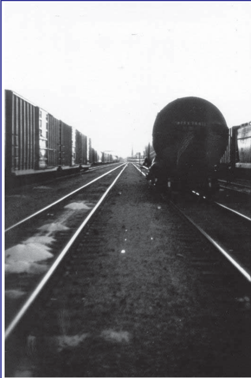
A railroad worker was killed by this tank-car, rolling silently downhill in a hump-yard. It was necessary to measure the contrast of tanker against the background to determine if the worker should have been able to see the car coming.
